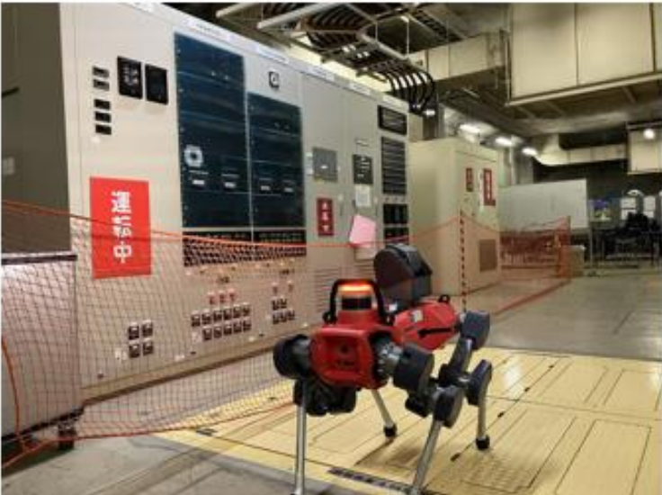
Quadruped patrol inspection robot (ANYmal)
