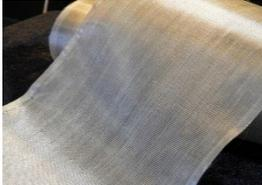
Production of high-performance long fibers from thermal power plant coal ash and commercialization efforts
