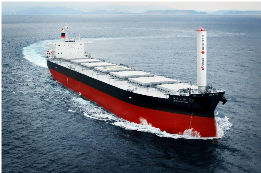
Image of the vessel equipped with the Norsepower Rotor Sails™
