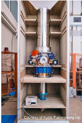
Gyrotron for heating plasma
