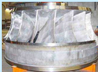
Tagokura Hydraulic Turbine Runner
