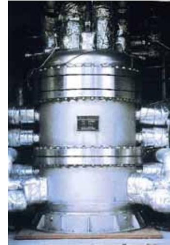
Solid oxide fuel cell (SOFC)
