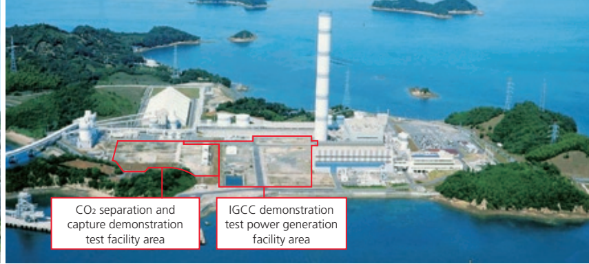
Planned layout of Osaki CoolGen test facility (Hiroshima Prefecture)
