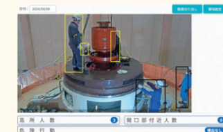
Display on a system screen when work in high places is detected
