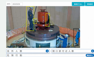
Display on a system screen when work in high places is detected
