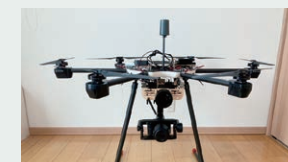
Transmission line inspection drone under development
