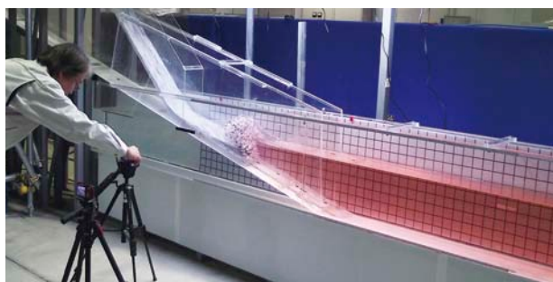
Experiment being conducted on water surface elevation due to an avalanche
