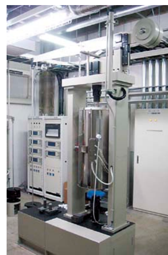
Large single-axis creep tester (maximum load of 200 kN) used to collect lifespan assessment data
