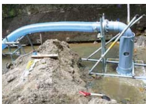
View of experiment in aspirating sediment
