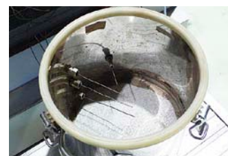
Air circulation tester used to assess spontaneous combustibility
