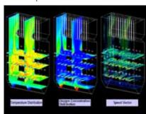
**Boiler Combustion Simulation Example**
