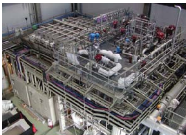
SOFC cogeneration system with an Atmospheric pressure (150 kw class) (Chigasaki Research Institute)
