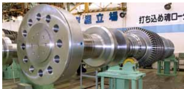
High- and intermediate-pressure turbine rotors at Matsuura Thermal Power Station (Nagasaki Prefecture)
