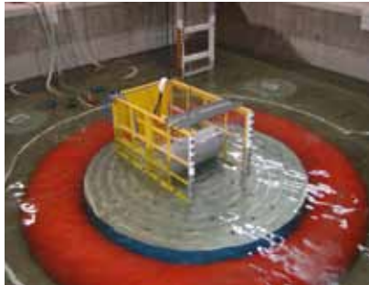
Vibration experiment using a large underwater vibration platform
