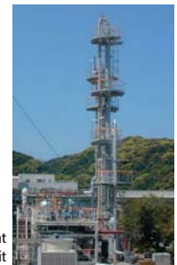
CO 2 separation and capture demonstration test equipment at the Matsushima Thermal Power Station No. 2 unit
