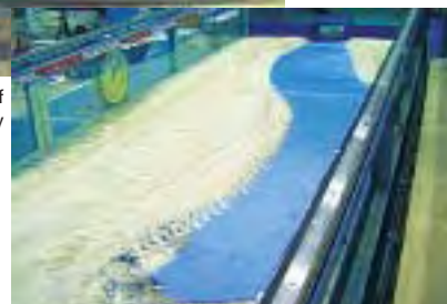
Hydraulic model test of sediment flushing technology
