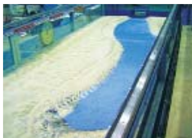
Hydraulic model flushing experiment
