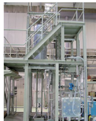
Electrically heated drop tube furnace (DTF) used to measure fuel combustion properties
