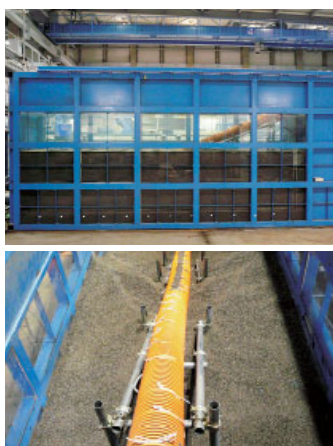
Experimenting with sucking in sediment by the sand aspirating and disposal method
