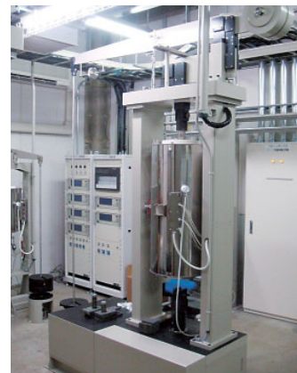
Large single-axis creep tester (maximum load of 200 kN) used to collect lifespan assessment data
