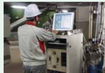
Field testing of new flue-gas monitor
