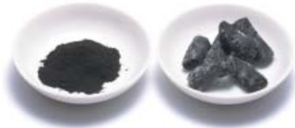
Carbon fuel from general waste Left: Carbon fuel made from general waste Right: Carbon fuel formed into briquettes for easy shipping and storage
