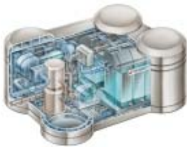
Normal-pressure SOFC cogeneration system (schematic diagram)
