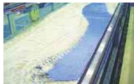
Bed-load transport experiment using hydraulic model
