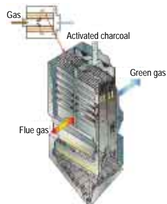
Dry type flue gas desulfurization unit (Desulfurization tower), Isogo Thermal Power Station
